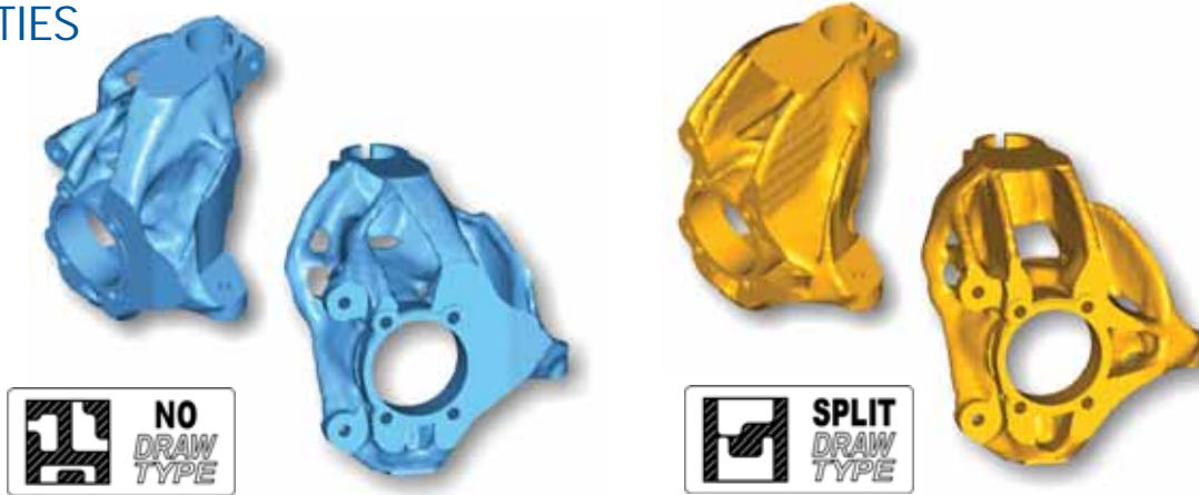
Applying Manufacturing Constraints Results in Feasible Knuckle Design
